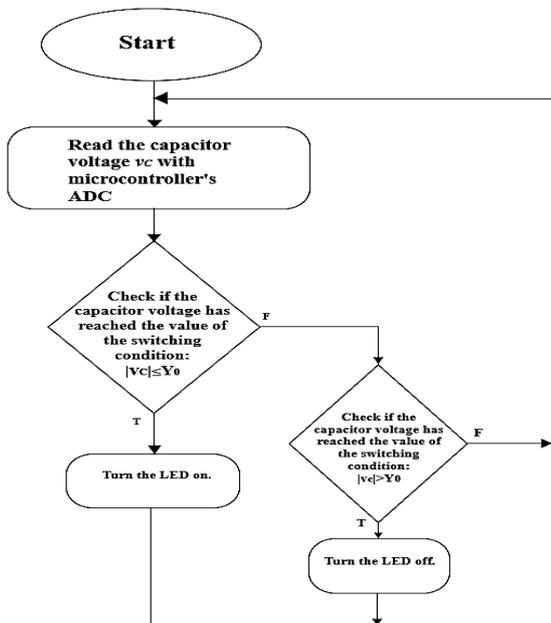
**Fig. 9.** The flowchart of the Biryukov oscillator program.
