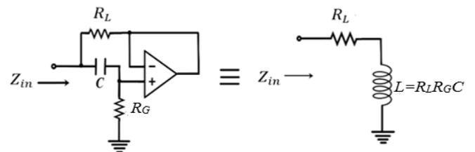
Fig. 7. The Gyrator circuit behaving as the inductor of the oscillator.
