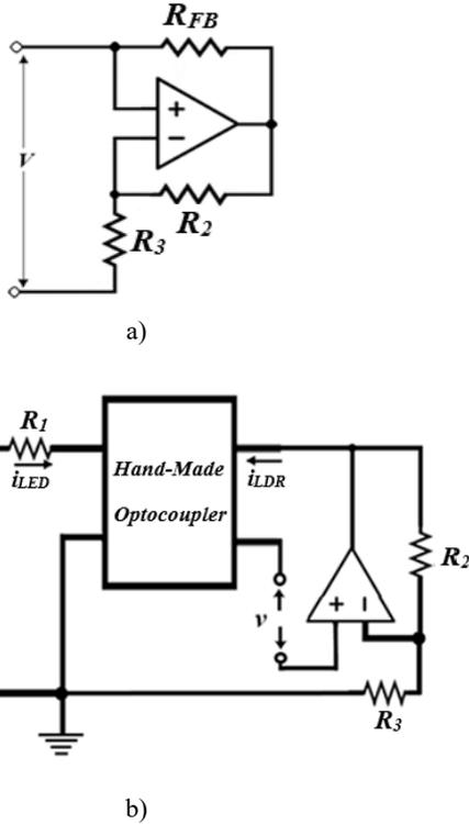
Fig. 5. a) The opamp-based negative resistor circuit and b) The modified negative resistor circuit of the oscillator.
