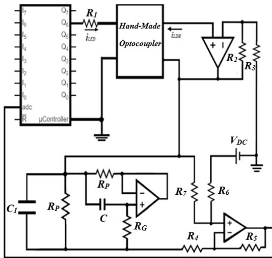
**Fig. 8.** The Biryukov oscillator circuit schematic
