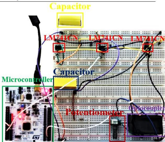
**Fig. 11.** Photograph of the implemented Biryukov oscillator circuit.
